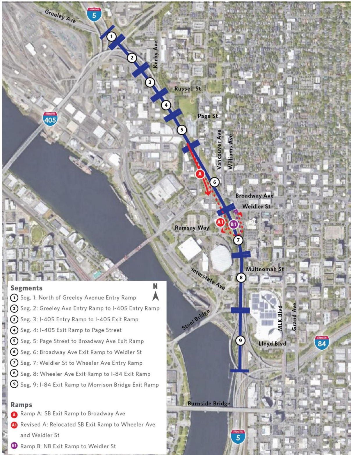
Figure 8 Study Segments and Ramps for Safety Analysis
