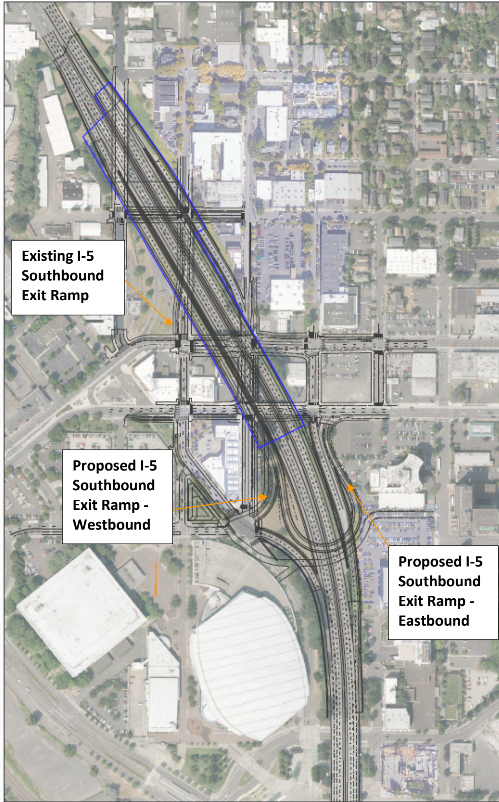
Figure 7 I-5 Southbound Ramp Relocation
