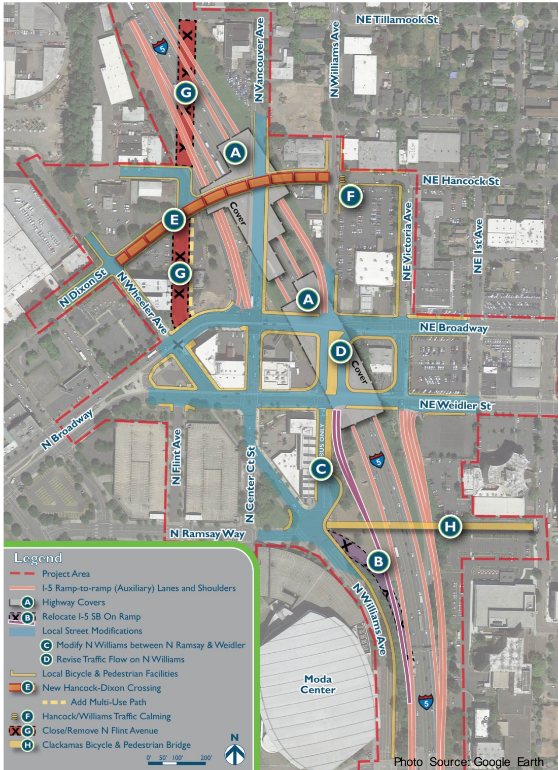
Figure 6. Broadway/Weidler Interchange Area Improvements
