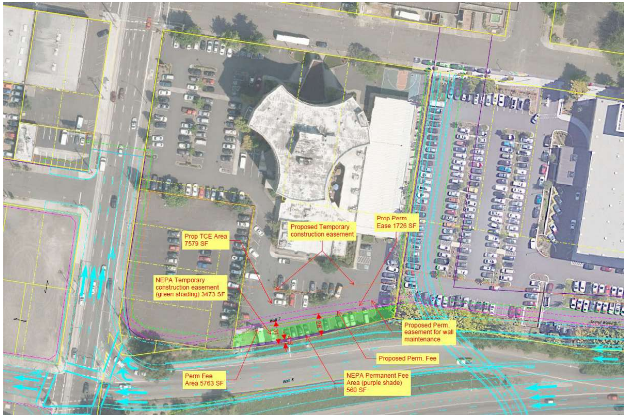
Right-of-Way needs for the Hybrid 3 design from the Travelodge at the Coliseum historic property.
