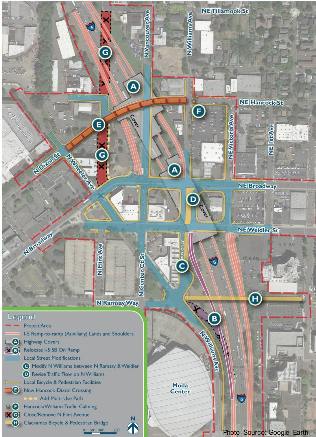
**Figure 7. Conceptual Illustration of Proposed N Williams Multi-Use Path and Revised Traffic Flow**
