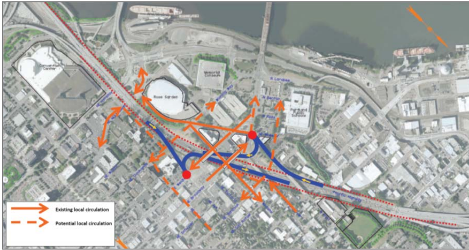
Figure 20: Example Concept (4b. Folded Diamond) for Phase II Analysis
