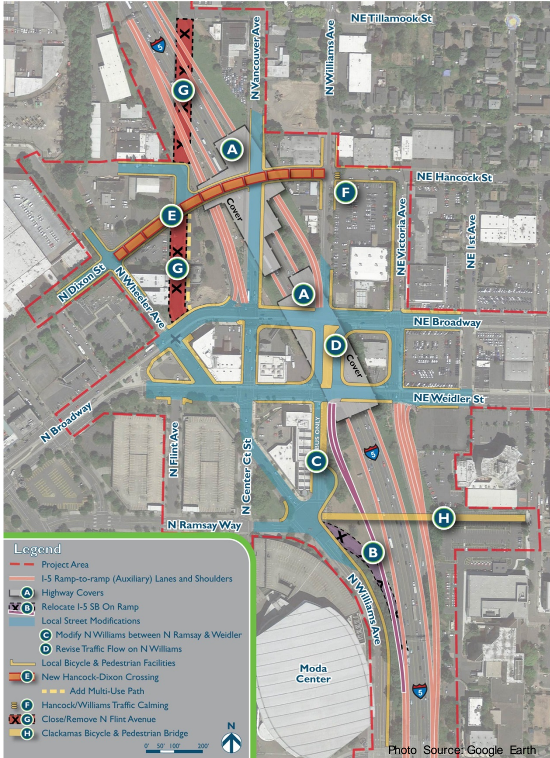
Figure 6. Broadway/Weidler Interchange Area Improvements
