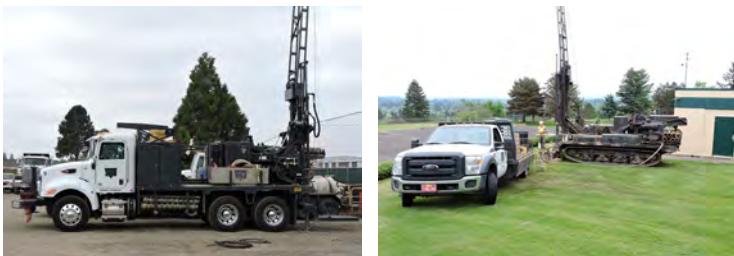
Truck-mounted rig used for soil sampling at most locations (left). Track-mounted rig used for soil sampling on sites with limited access (right).
