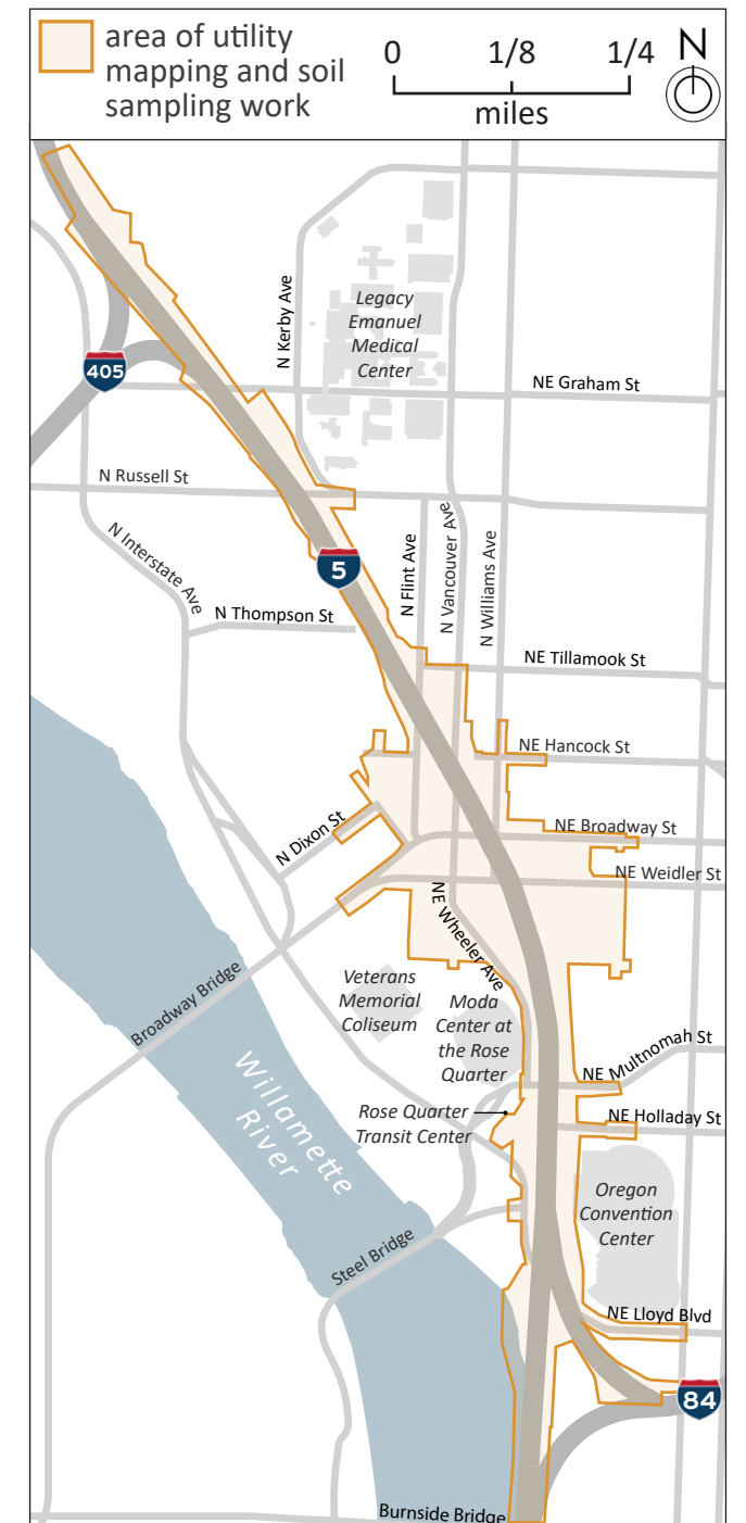
Soil sampling and utility investigation work will take place throughout the 1.8 mile-long project corridor, including some locations in the Willamette River.
