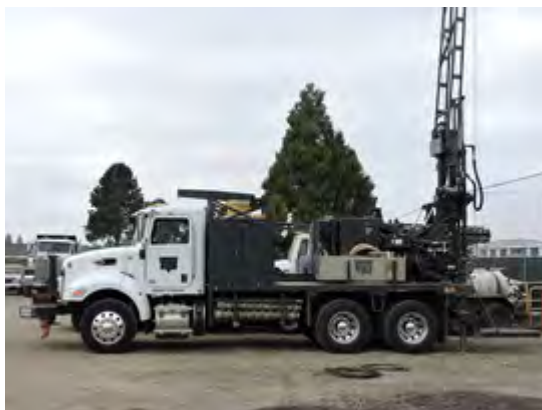
Truck-mounted rig used for soil sampling at most locations.
