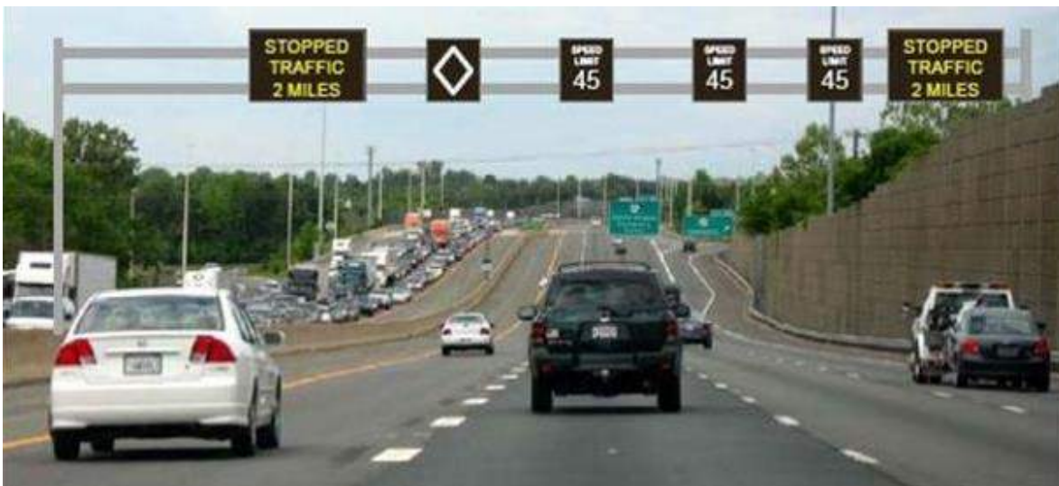
Figure 21 Matrix Signal, example from I-66 in Fairfax, VA
