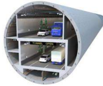
Alaskan Way Tunnel, WA 12' Lanes 2' Inside Shoulder 8' Outside Shoulder
