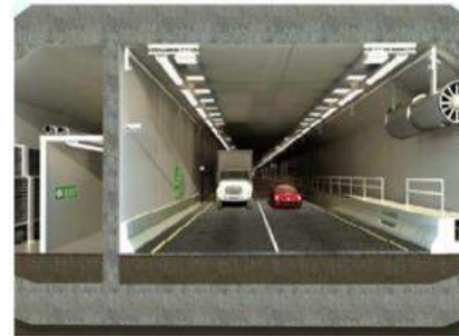
Midtown Tunnel, VA 12' Lanes 2' Inside Shoulder 2' Outside Shoulder
