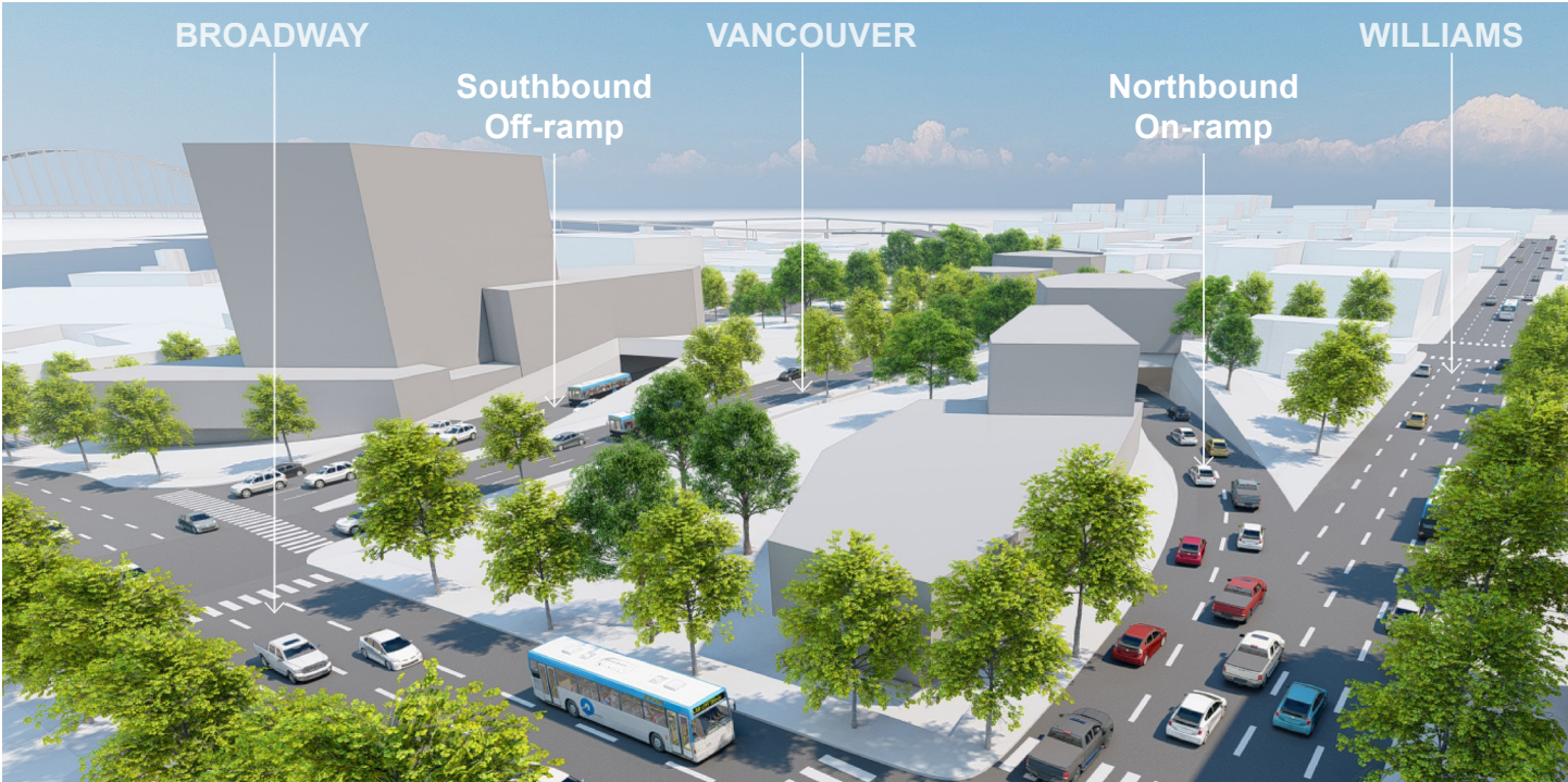
Figure 4: Conceptual rendering of Scenario 1. When rebuilt in their existing location, ramps create wide intersections, irregular parcels, and occupy valuable real estate that could have housed businesses and institutions.
