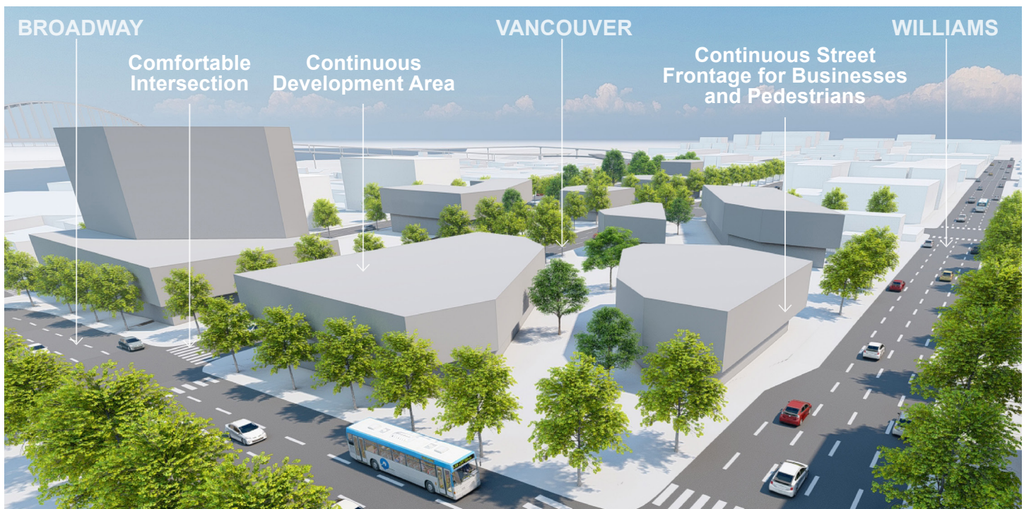
Figure 5: Conceptual rendering of Scenario 5. When ramps are moved south of the highway cover, the highway cover provides a higher quality urban environment with continuous street frontages, greater development area, and smaller, more comfortable intersections.
